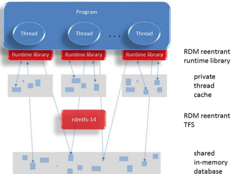
Figure 7: Single-Process, Multiple Thread Configuration
